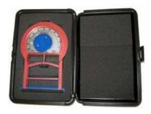
**Grip Strength device.** The Smedley III Analog Grip Tester is the most widely used hand dynamometer in the world for measuring grip strength. It is the most accurate with an accuracy of +/- 2 kg from 5 to 100 kg with a resolution of 1 kg. Holds the highest reading with an easily resettable pointer. The pointer is protected beneath the lens. Very durable and reliable. Includes padded hard case for easy, safe transport.
